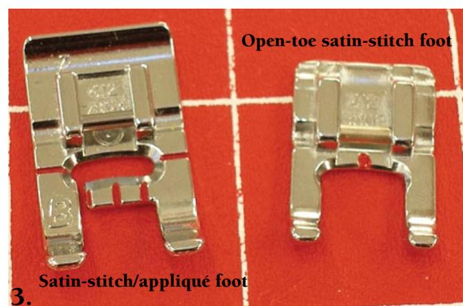
the needle window (the cut-out in the foot where the needle penetrates the fabric) and the underside of the foot. These sorts of stitches can have multiple layers of threads on top of each other to create the pattern, so the tunnel on the underside helps them form.
