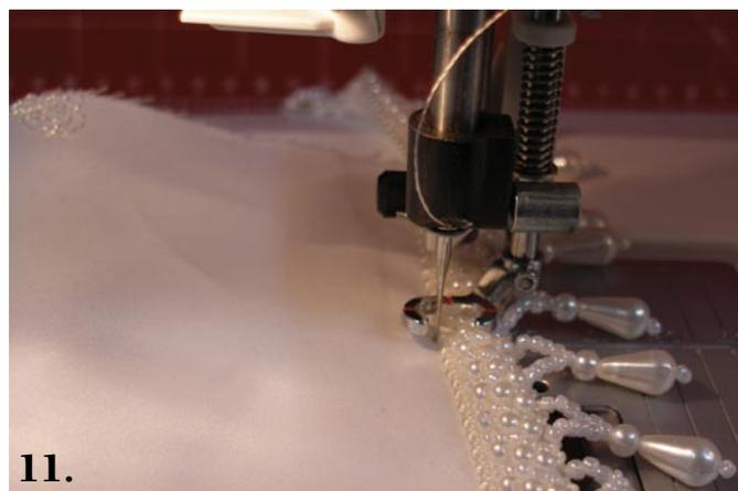
with the foot. When first using this foot for basting it seems very cumbersome, but with practice it's very easy, but remember to hold the threads to start with as they tend to want to pull out as the fabric is moving along.
